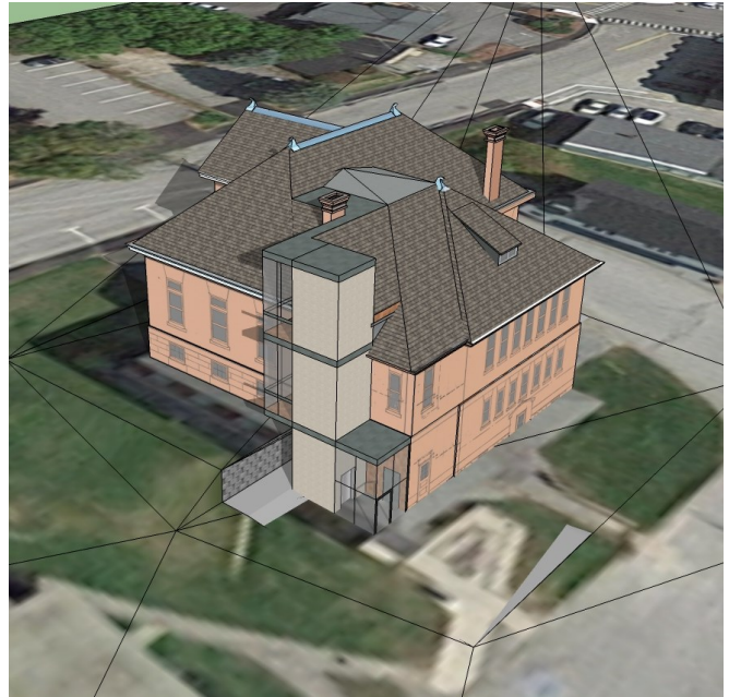
Preferred Option: New elevator placed outside building on West side of building.
